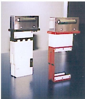
C Controlled-rate freezer (CRF) and retrieval module
