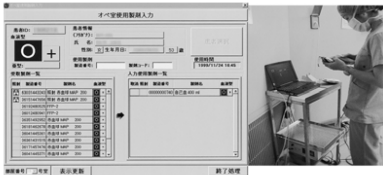
Fig. 4 Verification of blood units using a bar code at each operating theater. Each operating theater has a notebook-sized computer as a client to verify unit-recipient identification using a bar code (right figure). The left figure is the screen display of a client computer showing the information of the recipient undergoing an operation at the operating theater. All blood units compatible with the recipient are listed in this display including their particulars, the state of irradiation, product number, blood type and unit type. Just prior to transfusion, each blood unit is verified by a bar code for unit-recipient identification to avoid transfusion errors. Only compatible and irradiated (in cases of red cell and platelet unit) blood units are accepted and moved from the left panel to the right. This information is transmitted to the host computer in the transfusion service by the computer network system to update the usage data of the blood product in real-time as shown in Fig. 5.
