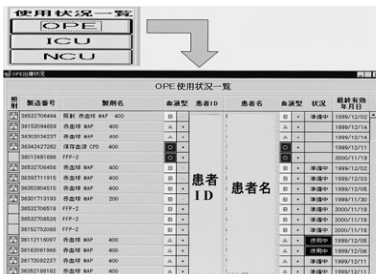
Fig. 5 Sample screen display of a client computer at the transfusion service monitoring the use of blood products in OPE, ICU and NCU in real-time via the computer network system described in Fig. 4.
