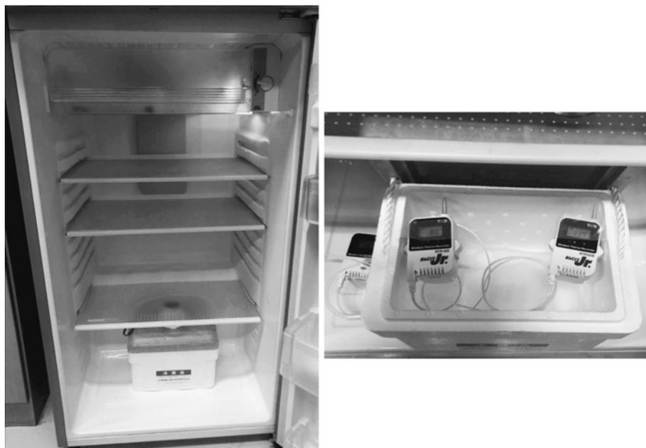
Fig. 5 Temperature inside a Styrofoam box and temperature inside a simulated blood bag in a domestic refrigerator
