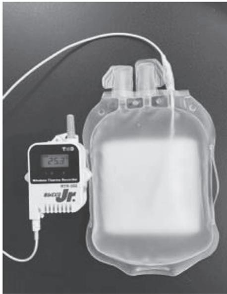
Fig. 1 Simulated bag and temperature wireless data logger
